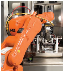
A TWO-AXIS OR MULTI-AXIS SERVO ROBOT CAN BE INTEGRATED INTO A SUNNEN MODULAR HONING SYSTEM.
